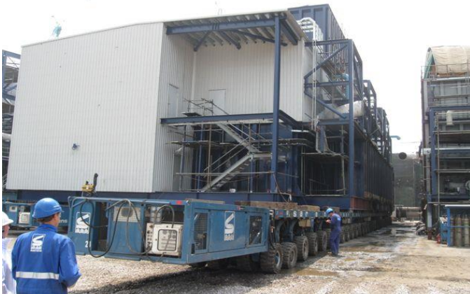
SWRO Skid Delivered to Pre-fabrication Yard
